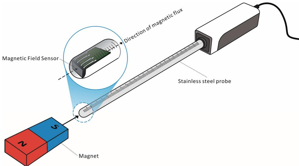
Figure 1. Measuring the magnetic field near a permanent magnet.
