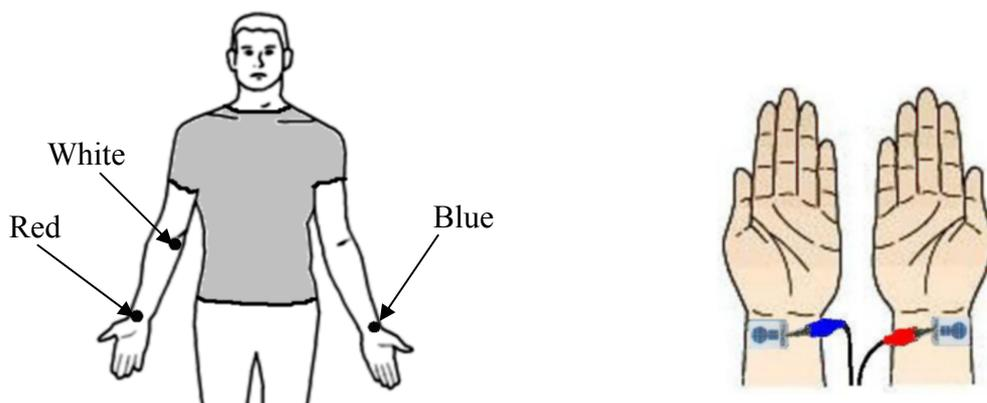
**Figure 3.** Connection of the ECG sensor to the body
