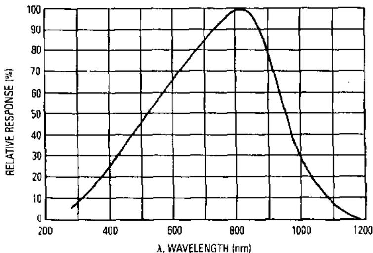
**Figure 3.** Relative spectral response of the Light sensor
