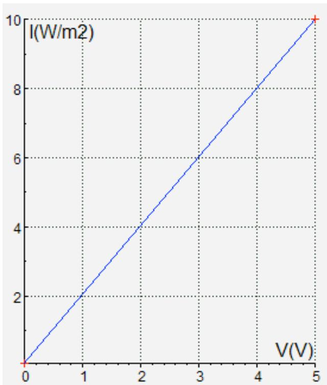
**Figure 2.** Calibration graph (range 0 .. 10 W/m<sup>2</sup>) of the Light sensor in the standard sensor library in the Coach program.
