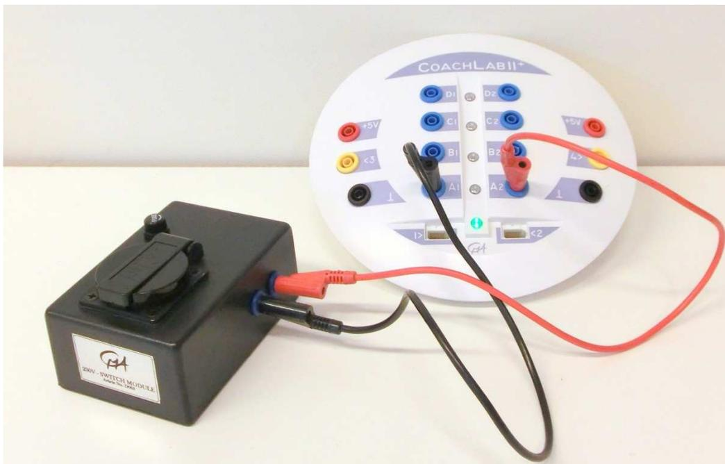
**Figure 2.** Connecting the switch module to the CoachLab II<sup>+</sup> interface.
